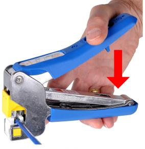
Remove the jack from the tool's receptacle.
