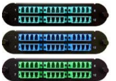
CCH™ Compatible LC 12 or 24 Fiber FPP-AD-LxQ-xx-C Available with internal shutters
