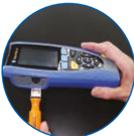
Replaceable RJ45 contacts
