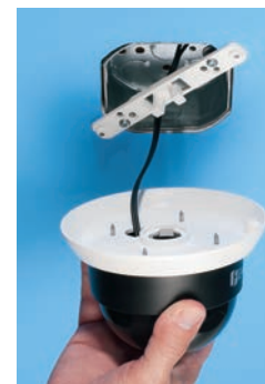
2 Place assembly on bracket. Turn clockwise to lock. Install set screw.
