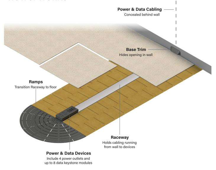
Total System Width: 34" Total System Height: .65" Maximum Raceway Length: 15' CONNECTRAC.
