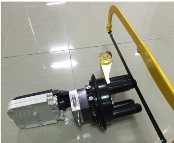
3. Saw off the cable ports from bottom by hacksaw
