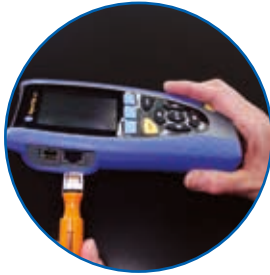
No calibration required plus replaceable RJ45 contacts
