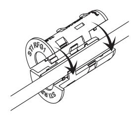
Install grommet halves around cable, teeth of grommets interlock securing grommet halves together.
