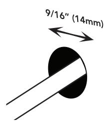
Cut nom. 9/16" (14 mm) diameter opening into gypsum board wall and run cable through opening.
