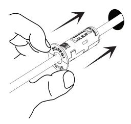
Slide grommet down cable into opening until faceplate abuts wall surface.
